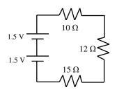
**Example**: Calculate the total resistance of this circuit.
